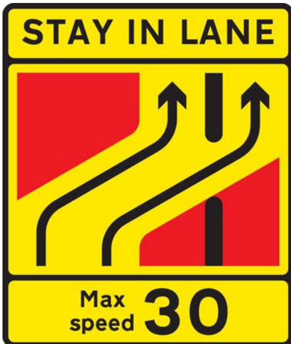
One lane crossover at contraflow road works
