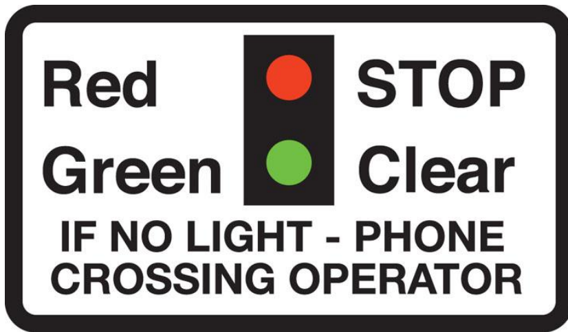
Miniature warning lights at level crossings
