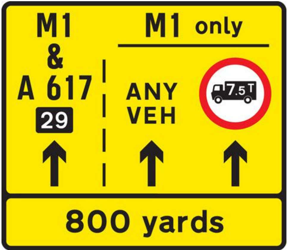
Lane restrictions at road works ahead
